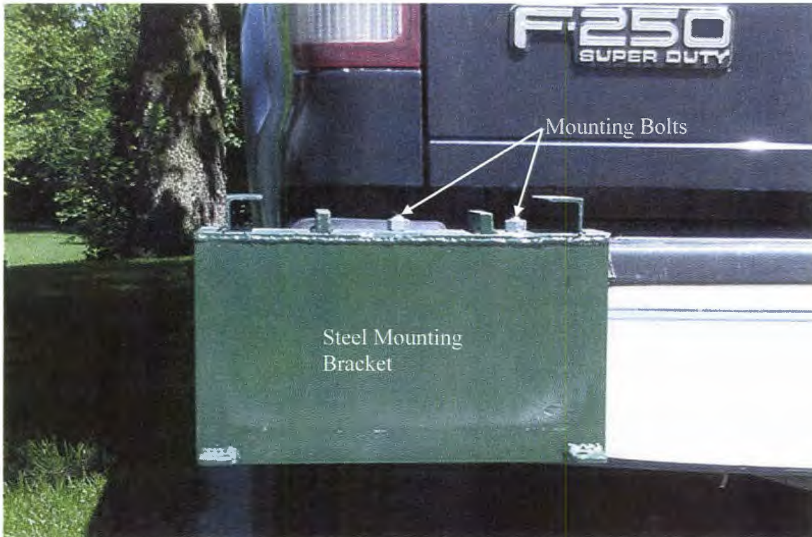
Figure 5.1.1. Steel mounting bracket and mounting bolts.
