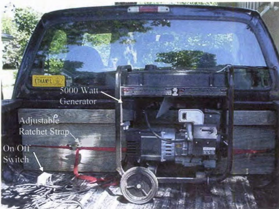
Figure 5.1.3. Generator secured by adjustable ratchet straps.
